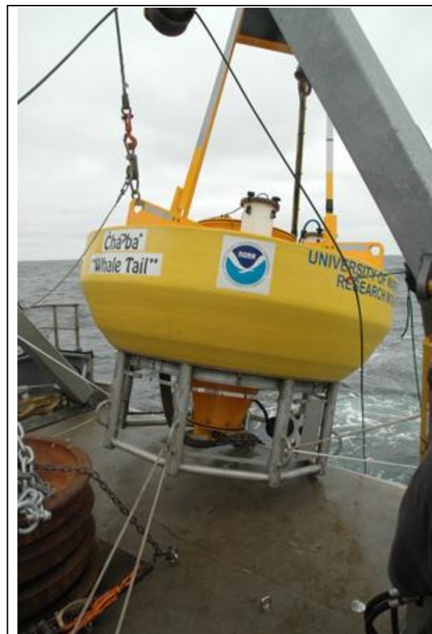
IOOS partners in the Northwest Association of Networked Ocean Observing Systems (NANOOS) deployed this buoy in 2010 as part of a three-piece observing array to assess issues in the Northwest, including ocean acidification , hypoxia and harmful algal blooms , and climate change . The coastal buoy will aid computer models that predict ocean and atmospheric conditions. Known as "Chá bã," the buoy is named for the Native American word (pronounced "chay buh") for "whale tail." (Photo courtesy of Dr. John Payne, Pacific Ocean Shelf Tracking Project.)
